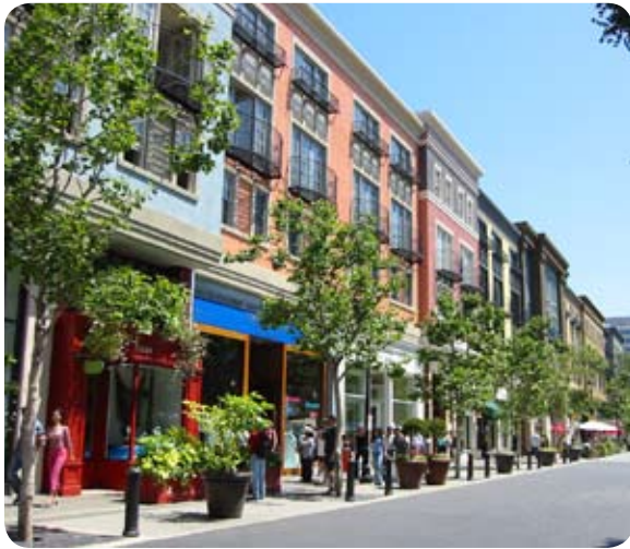
Figure 5.4.5 A strong cornice treatment separates commercial uses on the ground floor from residential above
