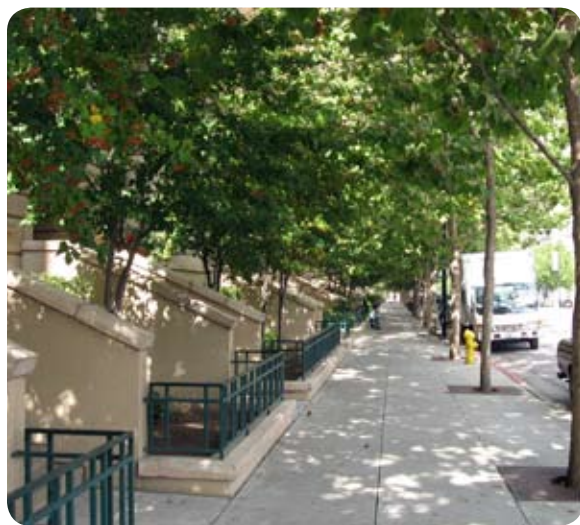
Figure 5.4.11 Stoops are a design technique used to separate public and private spaces
