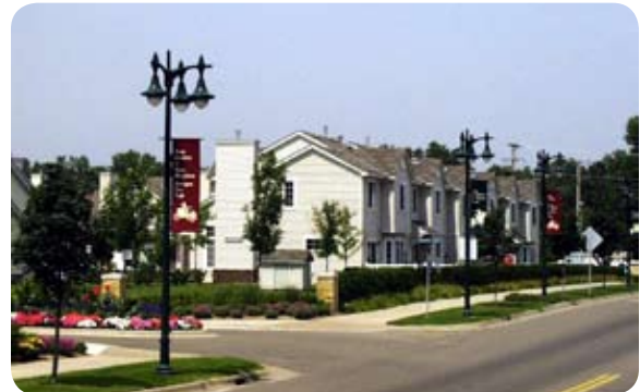
Figure 8.3.23 The spacing of lights depends on the level of pedestrian traffic
