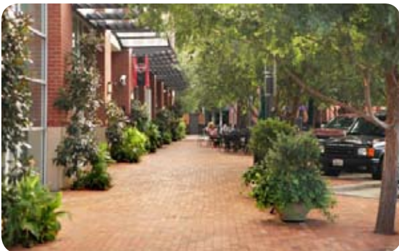
Figure 8.3.2 A sidewalk featuring a wide “through pedestrian zone”
