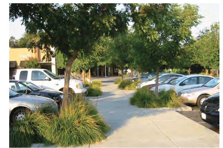
The use of shade trees and highly reflective paving can help to reduce heat gain in parking areas.
