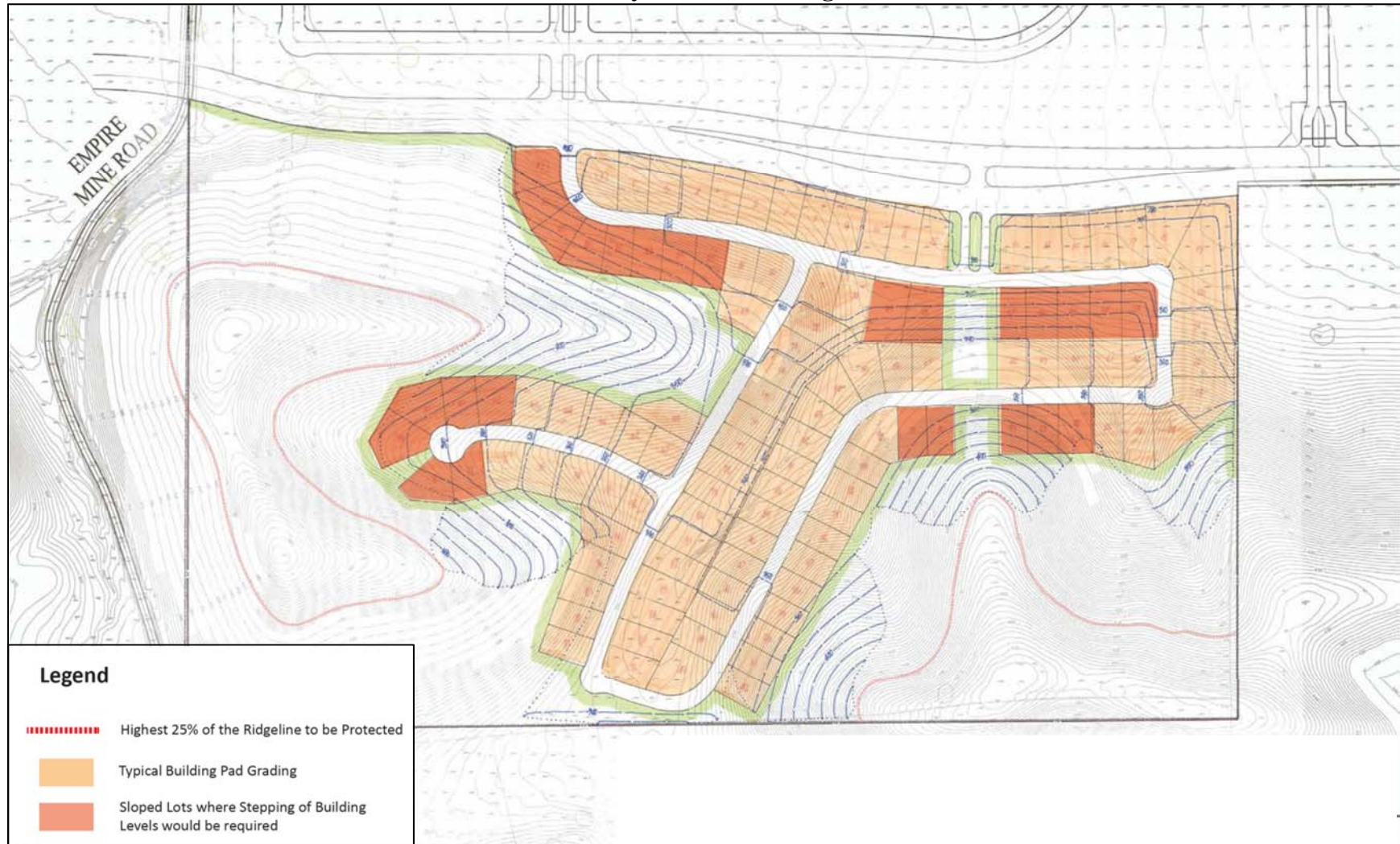
Figure 4.6-1 Preliminary Hillside Grading Plan
