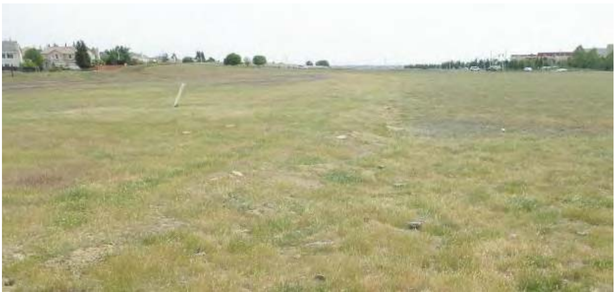
Photo 6: Seasonal Wetland Pool 1 at center right is located in native topography and soils. To the left of the pool is a raised grade of fill that has created an earthen dam resulting in the creation of this pool.
