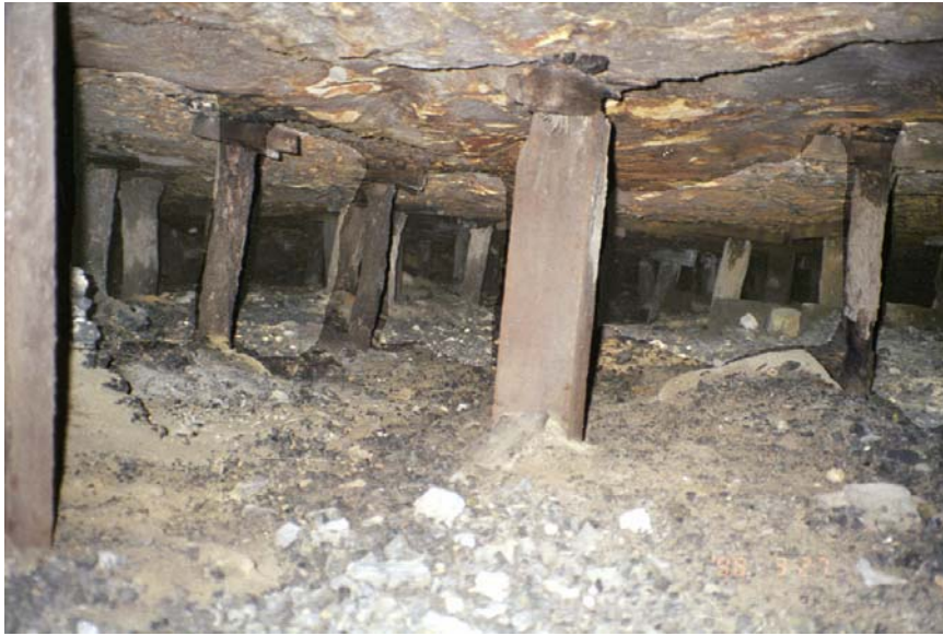
Photo 1: Looking down the dip of a mined out room. The wooden posts provide local support for the roof. They do not support the overall mined area. This area was mined more than 100 years ago.
