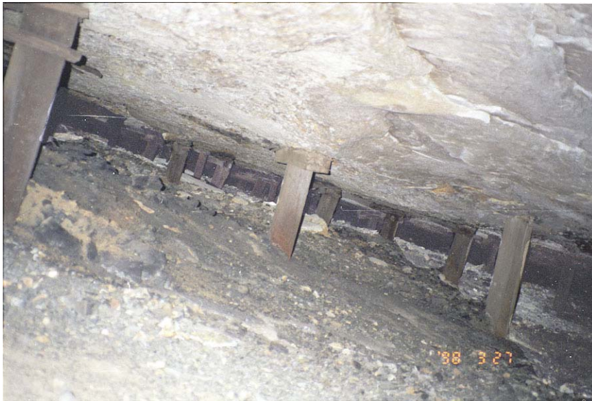
Photo 2: This is a view across a room with the camera kept level. It provides an indication of the dip of the coal seam.
