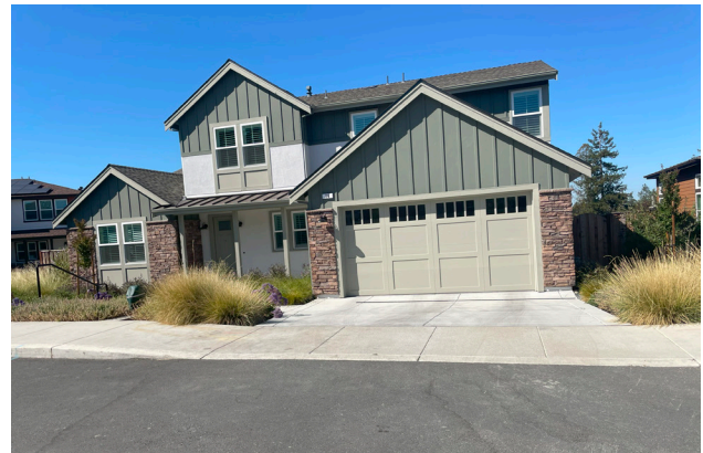
Front garage with sensitive design features such as proportional width and recess from surrounding wall plane.
