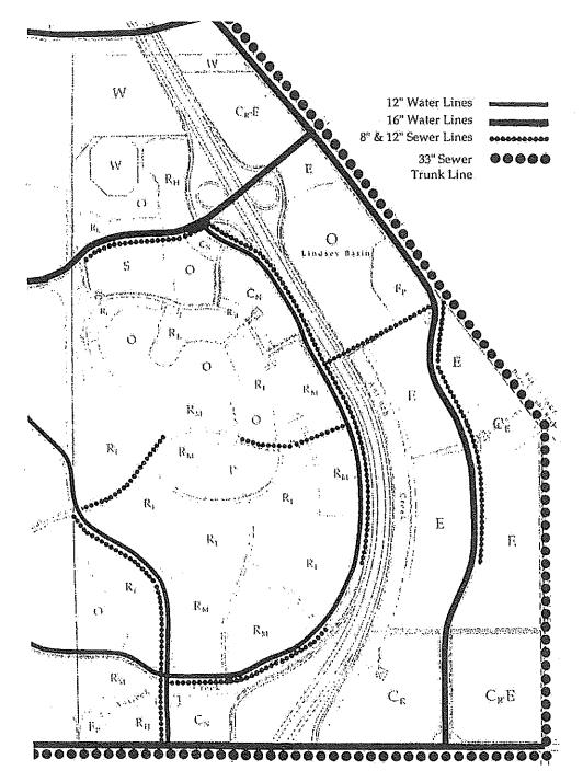
Figure 6.0. Water & Sewer Plan.
