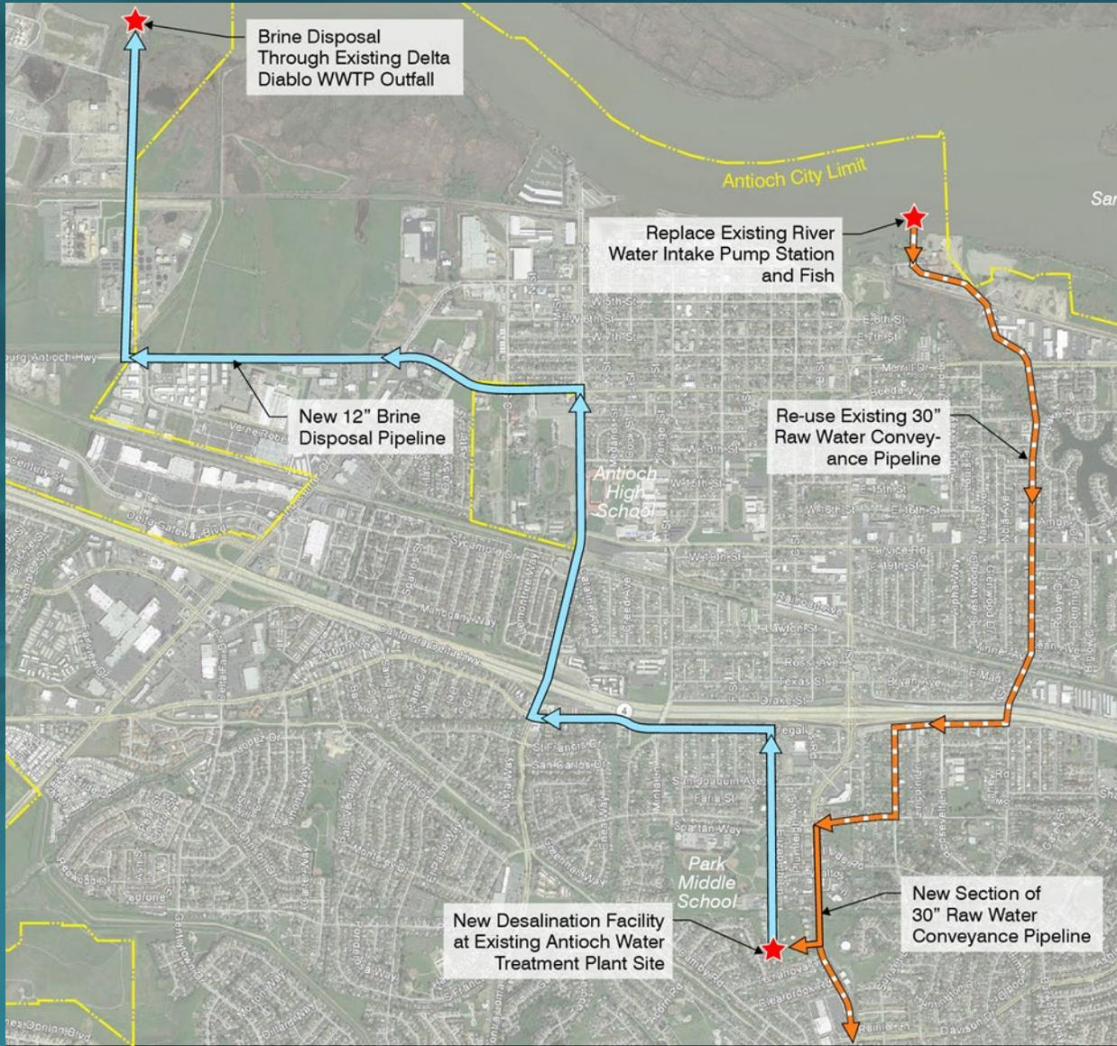
The Project will utilize reverse osmosis technology to enable the City to produce 6MGD of drinking water when Delta salinity is too high for conventional treatment
