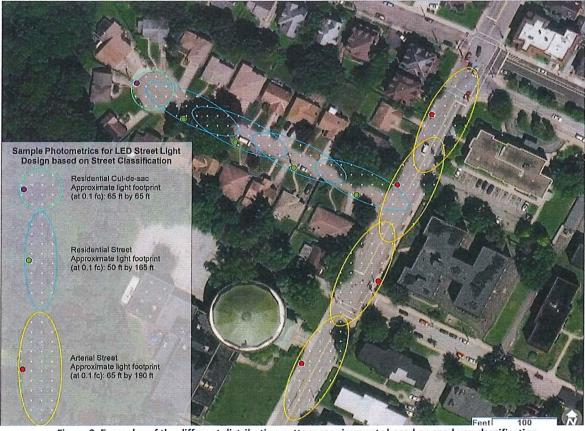
Figure 2: Examples of the different distribution pattern requirements based on roadway classification.
