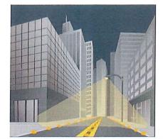
The dotted lines in the graphic above represent our method – which collects light measurements from significantly more locations – providing a comprehensive understanding of the fixture's light distribution pattern and photopic/scotopic performance.
