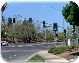
Project Description: This project will improve signal hardware including lenses, backplates with retroflective borders, mounting, size, and number. This will also install pedestrian countdown signal heads and install an advance stop bar before cross walk.
