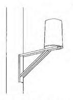
Drum-style antenna 24 to 26 inches high, 16 to 20 inches in diameter
