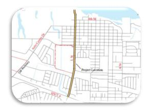
Project Description: The project will consist of construction of new sidewalks under the railroad tracks and along the fairgrounds, install curb ramps and re-striping to allow for complete bike lanes from HWY 4 to the Antioch Marina.
